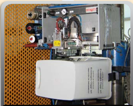
Coditherm Roller, for direct printing onto containers.
